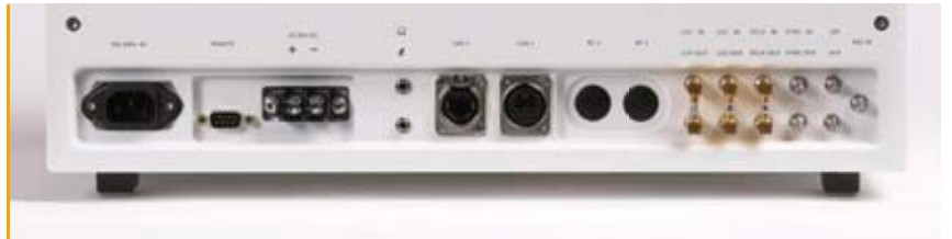
figure 7: External interfaces for power supply, LAN, GPS antenna and synchronization
