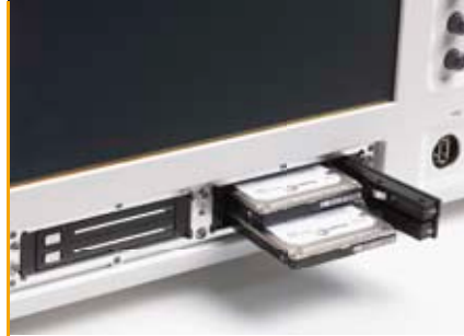
figure 5: Easy RAID storage swapping
